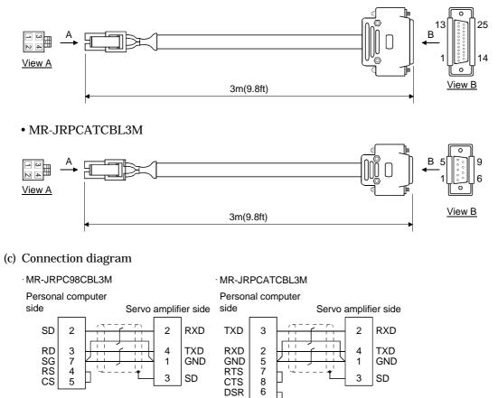
Note: The PC98 Notes having the connector of half-pitch 14 pins are also available. Confirm the shape of the RS-232C connector of the personal computer used.
